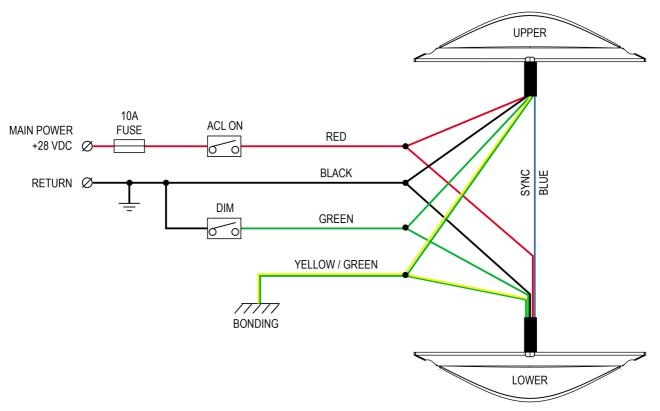
Note: When the light is dimmed, the intensity is not as required for flight operation. The installer must make sure the dimming function is switched off for flight operation. The light is designed that in case of a failure on the dimming circuit, the light will turn to bright and therefore be compliant to the regulation.
