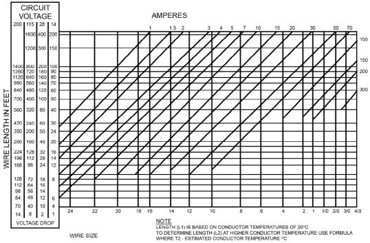
VOLTAGE DROP CHART INTERMITTENT FLOW AT 20° TIN-PLATED MIL-W-27759 CONDUCTOR
